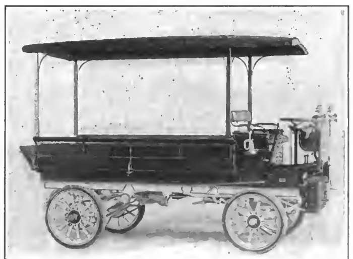
PACKARD TRUCK WITH 2-CYLINDER VERTICAL MOTOR
